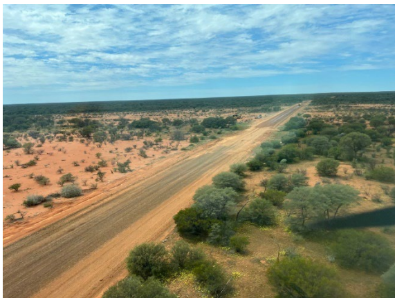
Rain shadow effect showing healthy thriving vegetation one side and rain starved vegetation on another caused by road levels and design.
